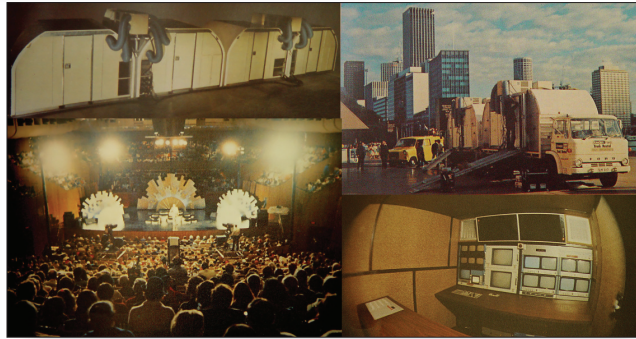
Figure 7.10 Here is a very unique "outside broadcast" system. Built for religious broadcaster Rex Humbard, the wheels used to get this system anywhere in the world included 747 landing gear. The system was built around four standard air-shipment modules, or "igloos," that would fit into a 747 fuselage used for cargo, since shipment via air was considered the most restrictive. The system also often traveled by ship — in fact, these photos are taken from a venue in Sydney immediately after a voyage through a typhoon, which dumped a couple of the containers on their sides. The final leg of the trip to the destination was usually via flatbed truck. The system supported three studio and three handheld cameras, along with three "quad" two-inch fixed VTRs and three portable quads. Each igloo had dimensions of seven by 10 feet, and was approximately seven feet high at the highest point, providing 440 cubic feet of space inside.
