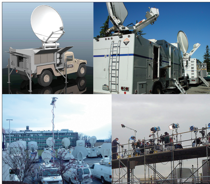
Figure 7.5 Production trucks come in lengths of less than 20 feet, and can even fit in a standard-size parking stall. The top two trucks allow multiple handheld cameras, often borrowed from the station's news department, to be used in small productions such as videotaped public affairs shows, and in some cases for commercial production, allowing the commercial spot to be edited on the spot and approved by the client. These trucks are designed so that only one person is needed, but they usually have provisions for two or three. The bottom two trucks have extendable masts for microwave transmission back to the station. These trucks often have modest production infrastructure, and sometimes can match the top two production trucks in production capability. Television stations might have both types of trucks if there is enough work for a microwaveless truck. Small trucks flourish because small means less: less money and simpler logistics for operation. (Source: Wolf Coach)
