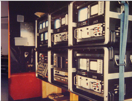
Figure 7.8 Flight cases can be used to turn a vehicle that usually has a different mission in life into a temporary remote vehicle. Here a snow cat is converted to a remote production vehicle for the 1984 Winter Olympics in Sarajevo by strapping flight cases into place. (Source: A.F. Associates)
